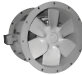
Marine Duct Axial®. Sizes 12" – 60". Up to 92,000 CFM, S.P. to 4". Series 44 M See bulletin A143*
