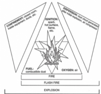
Diagram shows the requirements for a fire, flash fire and an explosion.
