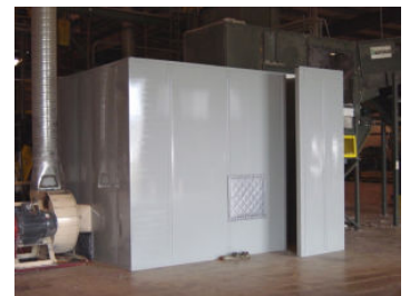
Rigid metal noise enclosure surrounding the hammermill that resulted in a 19 dBA reduction of noise levels within the facility.
