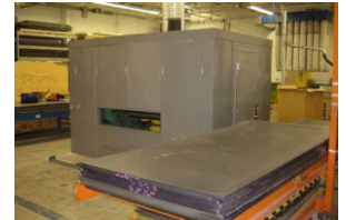
Acoustic enclosure implemented to decrease noise levels created by an industrial planer.
