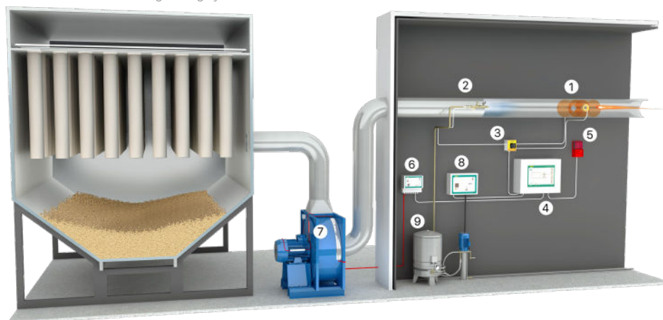
Mounting principle of the spark detection and fire extinguishing system
