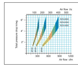
The black line shows the pressure drop for the extractor when in the same position as the arm on the design above. The area in the diagram shows the pressure drop at normal use. The different tints show air velocity in the extractor according to the code below. Recommended transport velocity for welding fumes is 3550 ft/m.
