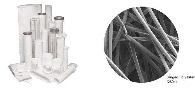
Needled 16 oz. singed polyester felt is a versatile and cost effective filtration media used in pulse jet baghouse dust collectors. The singeing process removes fiber fuzz and creates a more uniform finish, allowing for a better dust cake release than untreated polyester media. This material is strong, abrasion and chemical resistant and good for applications up to 275° F.
