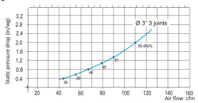
The static pressure drop is measured in accordance with ISO-standard 5167-1. The noise level is measured in accordance with ISO-standard 3741.
