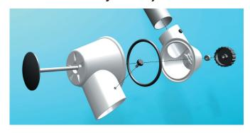
**Terfu joint.** The large frictional diameter together with the single grip adjusting knob provide a rigid, stable joint with a smooth easily adjustable function without requiring the application of excessive force or tools. The joint has reinforced side pieces. Ball bearings that isolate the adjusted friction level allow the arm to move up and down without locking the joint or loosing stability and function.
